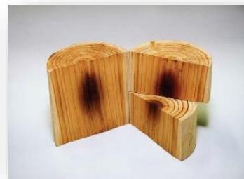
Picture 4 - Microwaves are heating from the inside out
