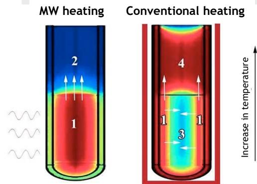
**Picture 8 - Microwave and conventional heating**
