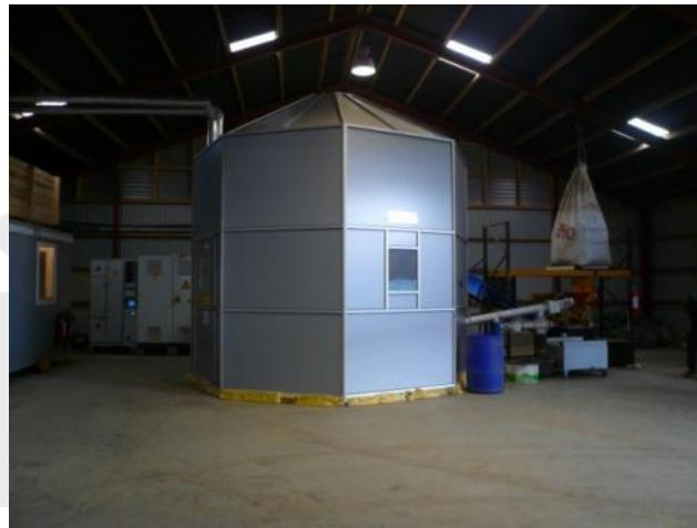
Picture 19 - the “octagon” protects the reactor and serves as an additional outer radiation shield
