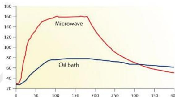
**Picture 7 - typical microwave heating curve compared to conventional heating**
