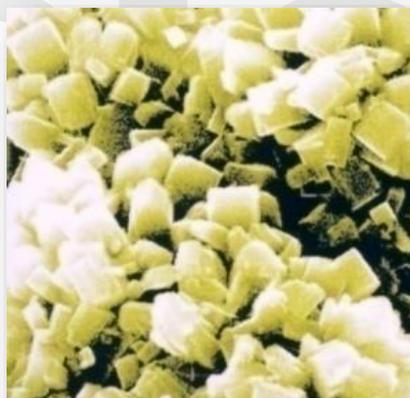
Picture 5 - Zeolite Catalyst under the microscope
