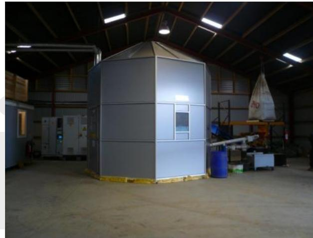
Picture 19 - the "octagon" protects the reactor and serves as an additional outer radiation shield
