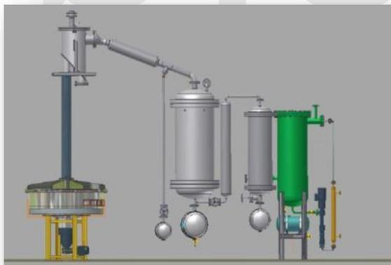
Picture 3 - Oil vapors emerging from the reactor are subsequently condensed and cleaned in a quencher unit
