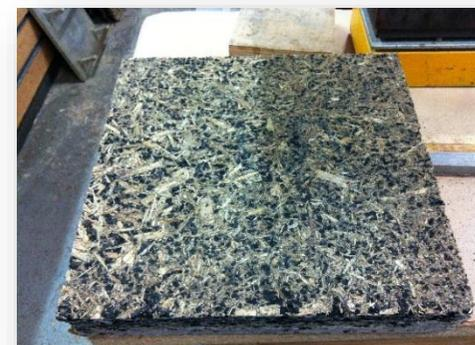
Picture 18: Pressboard with 60%  $\mu$ Char
