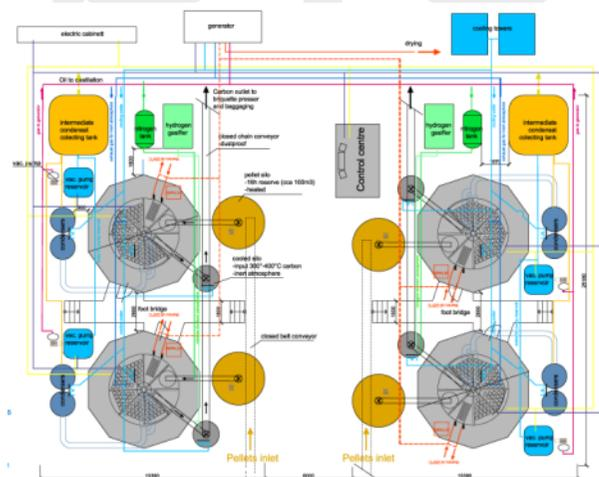
Picture 12 - A 4xcluster floor plan
