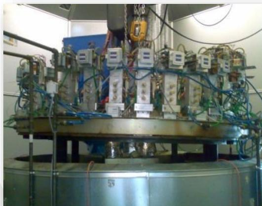
Picture 4 - A pilot reactor opened up for inside maintenance
